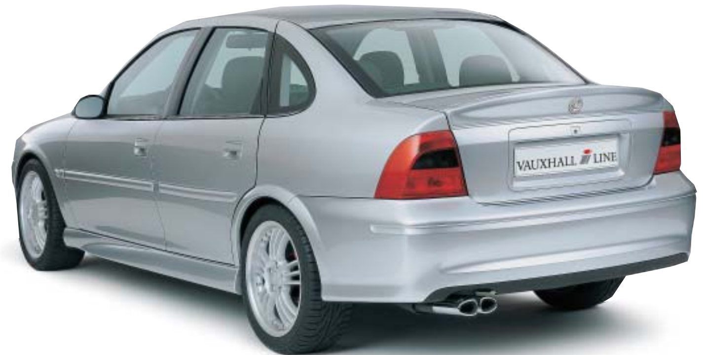
Rear lip spoiler (from My. 99,5) i 29 01 422, side sills (from My. 99,5) i 29 01 319, rear silencer (from My. 99,5) i 29 08 045, light alloy wheels in Spectra Sports Line design.
